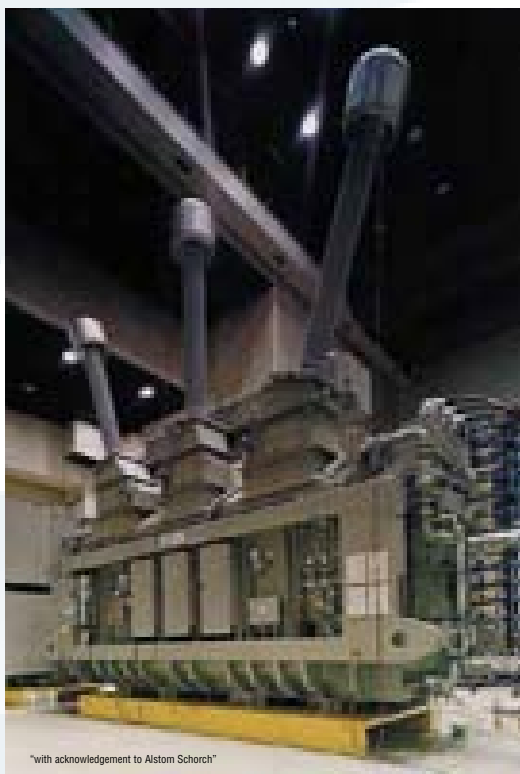
420kV & 123kV oil insulated transformer bushings with composite insulators
