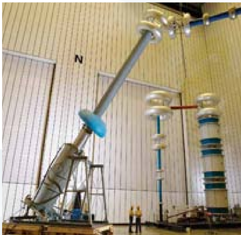
800kV Extra HVDC Transmission Bushing
